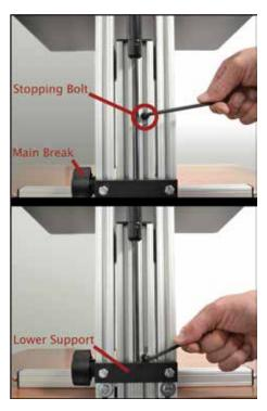
On the back side of your unit you will notice a small bolt located on the lifting tower. This bolt is used as our work surface stopper. It is currently set at 15", the highest our unit should go. This setting is for a 6'2" user on a 30" high desk. If you are shorter than this, raise the unit to your desired height and tighten the Main Brake. Adjust the stopping bolt by loosening the bolt with one turn and drop the bolt down to reach the lower support, and re-tighten the stopping bolt.
