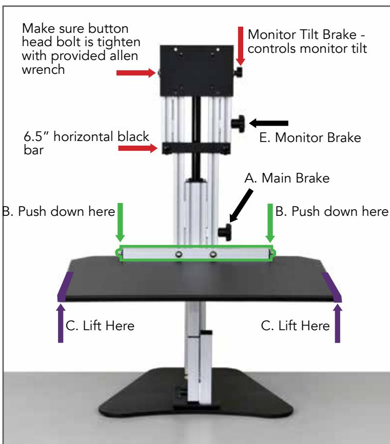
To raise the Pro Junior, loosen the main brake(A) and lift the main work surface on the sides(C & C). Once you have the work surface at the required height tighten the main brake.
