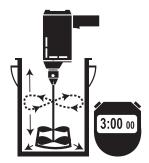
specified. Using a low-speed drill and Jiffy Mixer, mix well from top to bottom and side-to-side for a minimum of 3 minutes before use. Avoid mixing air into the product.
