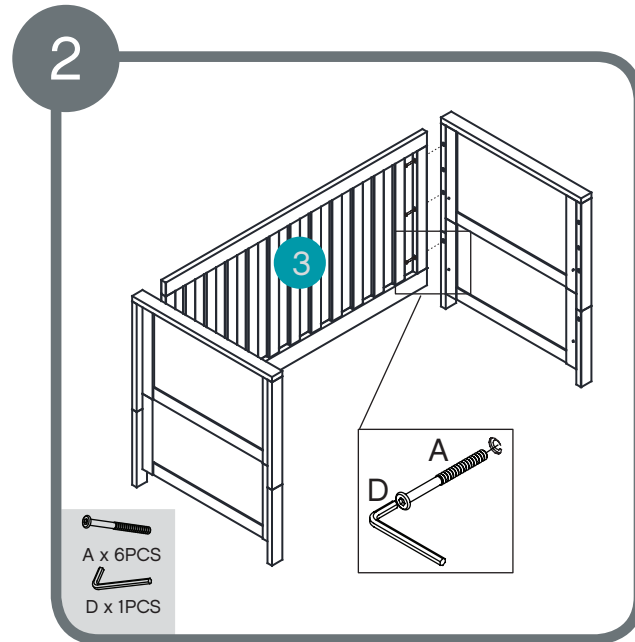
Assemble side using 6 x A bolts
