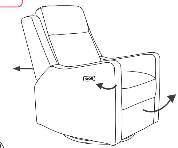
**CAUTION:** Do not allow children to play on this electronic chair or operate the mechanism. The leg rest folds down on closing and could possibly injure a child if they are near the folding mechanism. Do not leave children unattended on or near the chair. Always leave the chair in an upright and closed position. Keep hands and feet clear of mechanism. Only the adult occupant should operate the chair.
