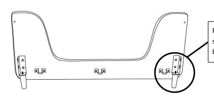
For the side Panels, use 4x M8 Screws to attach the 2x side brackets and 8xM6 Screws to attach the 3xsupport brackets into the side panel.
