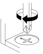
Turn cam lock clockwise to tighten.
