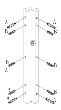
No. A Quantity:16 Pcs Cam Lock Dowel 8\*28mm No. B Quantity:24 Pcs Dowel 8\*30mm
