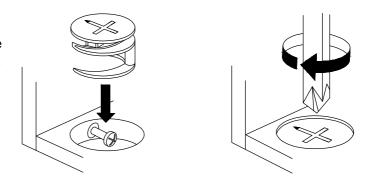
Turn cam lock clockwise to tighten.
