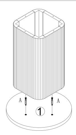
No. B Quantity:4 Pcs Cam Lock Dowel 8\*28mm
