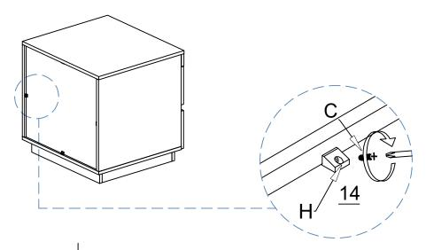
No.H Quantity:4Pcs Back Plate Clamp No.C Quantity:4Pcs Screw M3.5\*14mm
