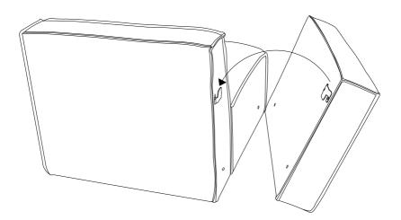
Ensure to attach the armrest in the right position and properly align the holes before screwing them in.
