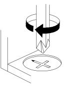
Turn cam lock clockwise to tighten.
