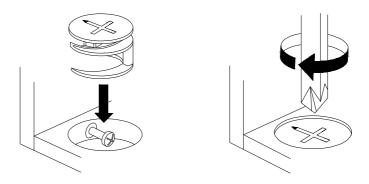
Turn cam lock clockwise to tighten.
