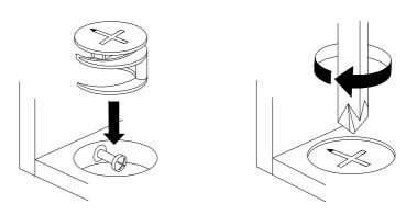
Turn cam lock clockwise to tighten.
