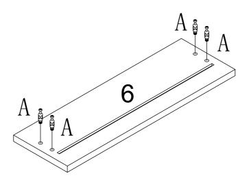
No. A Quantity:4Pcs Cam Lock Dowel 8\*28mm
