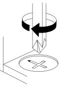
Turn cam lock clockwise to tighten.
