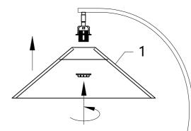
Twist out the plastic ring on the lampholder, install the shade, then install the shade, tighten the plastic ring back.
