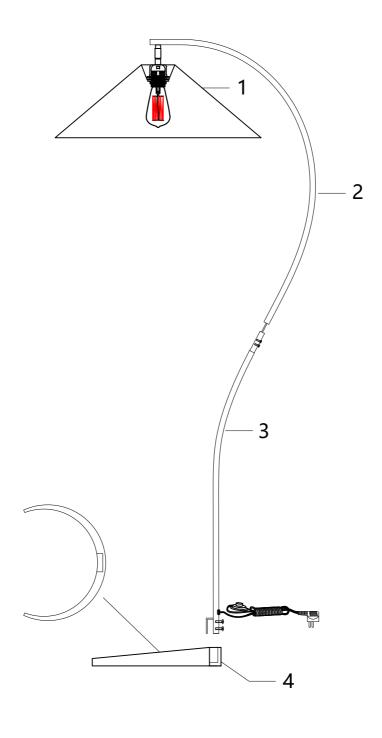
Unscrew the screws on upper of the bending tube 3, then insert the tube 2, fasten back by the screws
