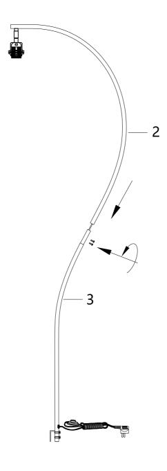
Pull out the supply cord a bit, unscrew the screws on the 3, then insert the part 2 into the 3, fasten by the screws.
