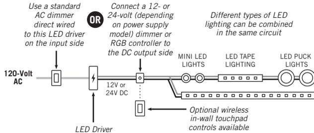
**Never combine a 120-volt AC dimmer, a 12/24-volt DC dimmer, or an RGB controller in the same circuit. Using a standard on/off wall switch with a 12/24-volt dimmer or controller is permitted.**
