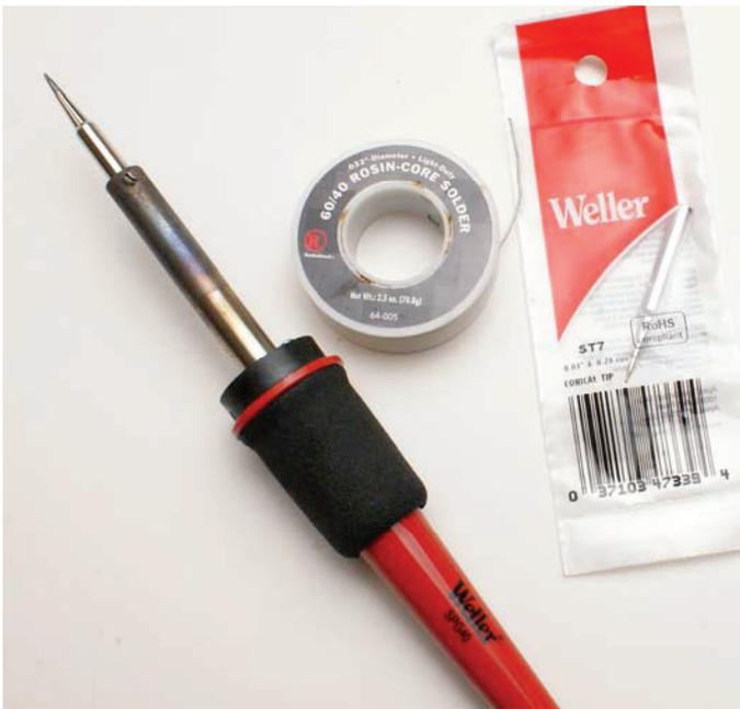
Use a fine point conical soldering tip. (Weller model ST7 shown below.)
