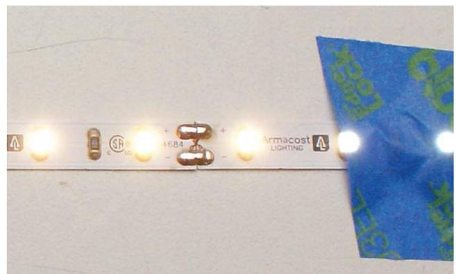
Be sure to power up your LED lighting prior to final installation. Check to ensure that all tape sections are lighting properly and connections are solid.
