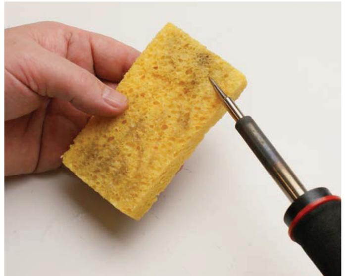
Use a wet sponge to remove excess solder and to keep tip clean. Soldering stations are also useful and readily available online. (Weller WLC 100 shown below.)
