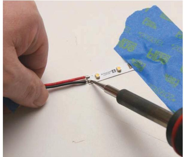
Once the wire leads and copper pads are tinned, join the wires to the copper pads and solder using a clean soldering tip. No extra solder is required since tinning has been done. Be sure to maintain correct polarity (+ to +, - to -, R to R, G to G, etc., depending on the type of tape light you're working with.
