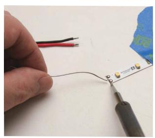
The same basic tinning process is also required on each of the copper pads on the LED tape lighting. Use painter's tape to secure the LED tape when you are soldering.
