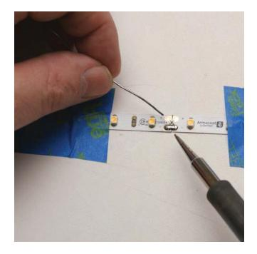
Next, tin each section of the copper pads with a small "mound" of solder. Then, with the tip of your hot soldering iron, drag one solder mound to the adjoining mound to form a single, continuous larger oval solder mound.
