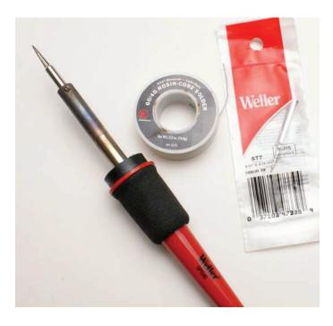
Use a fine point conical soldering tip. (Weller model ST7 shown below.)
