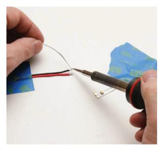
When soldering power wires to LED tape, first prepare the wire by "tinning" the stripped ends of each wire lead. Place the tip of the hot soldering iron against the wire and apply a light, even coat of solder as shown.
