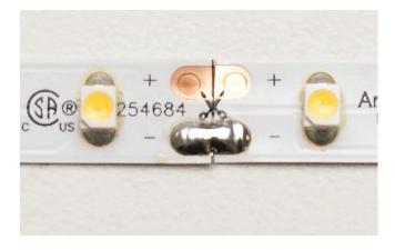
Repeat for each copper pad connection. Done properly, the soldered splice connection will be as strong, and last as long, as any factory-made connection.
