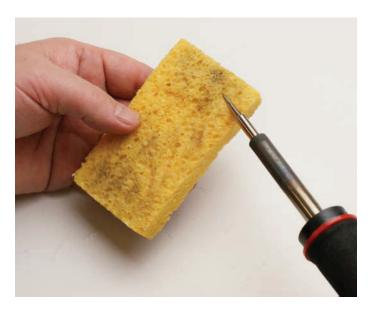
Use a wet sponge to remove excess solder and to keep tip clean. Soldering stations are also useful and readily available online. (Weller WLC 100 shown below.)
