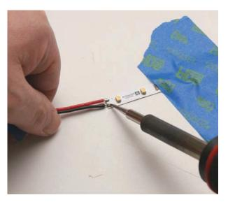
Once the wire leads and copper pads are tinned, join the wires to the copper pads and solder using a clean soldering tip. No extra solder is required since tinning has been done. Be sure to maintain correct polarity (+ to +, - to -, R to R, G to G, etc., depending on the type of tape light you're working with.
