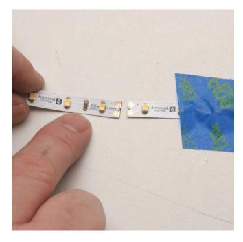
Maintaining polarity with the tape lighting, join together two sections on a flat surface as shown. Secure the LED tape in place with painter's tape.
