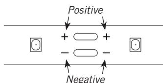
**NOTE:** Be sure all 12-volt connections are secure and protected from electrical shorting. Options include electrical tape, small wire nuts, crimp connectors, etc.
