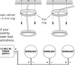
On very large, multi-LED light installations, be aware of possible voltage drop, which only becomes undesirable if you notice the brightness in one area of your lighting is objectionably different than in another area. Do not coil wire; shorter lengths and thicker wire will mean less voltage drop and higher brightness. For an online voltage drop calculator, visit armacostlighting.com/voltagedrop.
