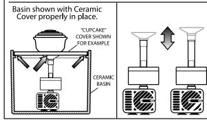
If necessary, adjust the height of the Top Seal by sliding it up or down on the Rigid Tube.
