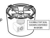
Place the Ceramic Cover onto the Ceramic Basin to check if any height adjustment is needed for the Top Seal on the Rigid Tube. Adjustment is needed if Ceramic Cover rocks back and forth due to interference with the Top Seal.
