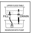
IMPORTANT: The DRAIN FITTING must <u>always</u> be larger than the FILL FITTING to allow sufficient draining of flood table to prevent overflow.
