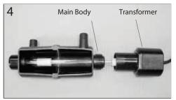
transformer into the quartz sleeve and screw the transformer onto the main body. Do not over-tighten! Hand tighten until snug. (See Photos 2, 3 & 4)
