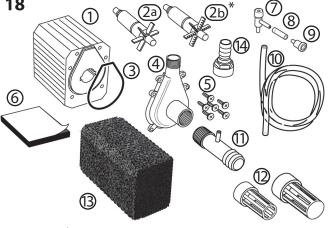
\* Note: Hydroponic models ship with Regular Impeller. Fractionating impeller can also be purchased separately and used to induce even finer bubbles into water stream.
