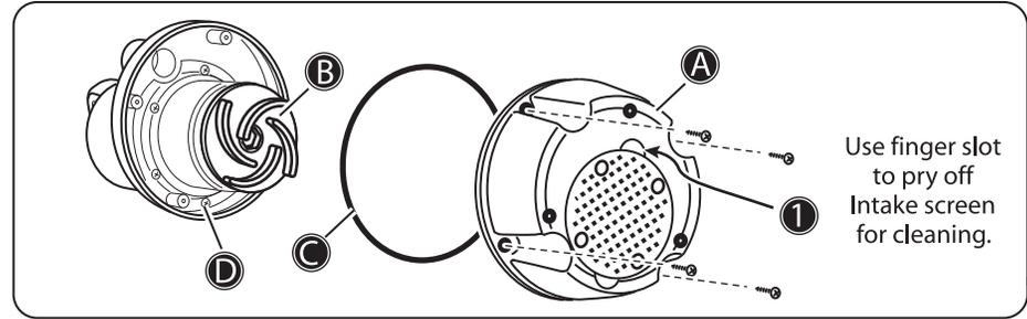
Periodically cleaning the impeller will maintain pump performance and extend pump life.
