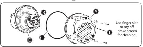
Periodically cleaning the impeller will maintain pump performance and extend pump life.
