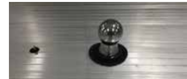
Image of Hide-A-Goose after installation.
