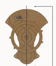
**Important:** Base must be mounted level as shown here so it will operate correctly.
