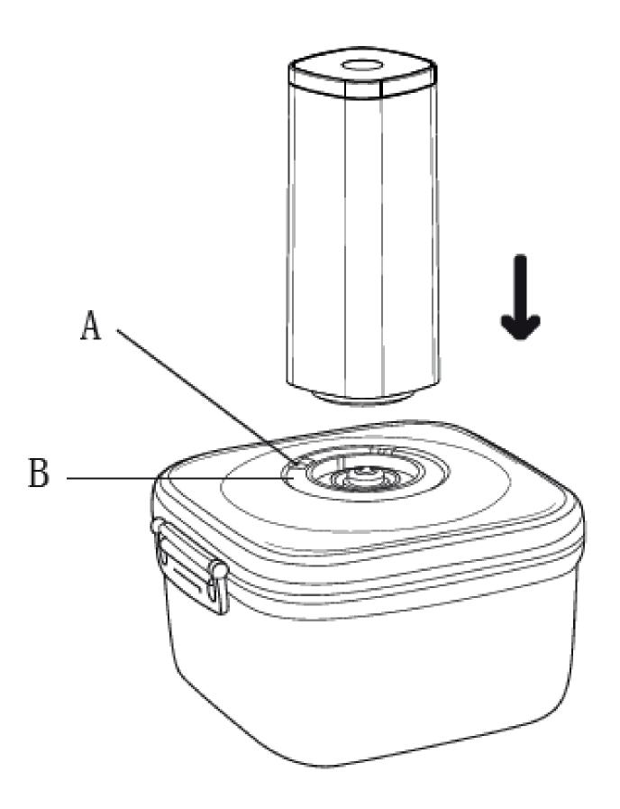
1. Place the pump in the middle of the valve. Press down the pump a bit. Push the button on the Pump. The pump pulls air out of the box untill vacuum is obtained.
