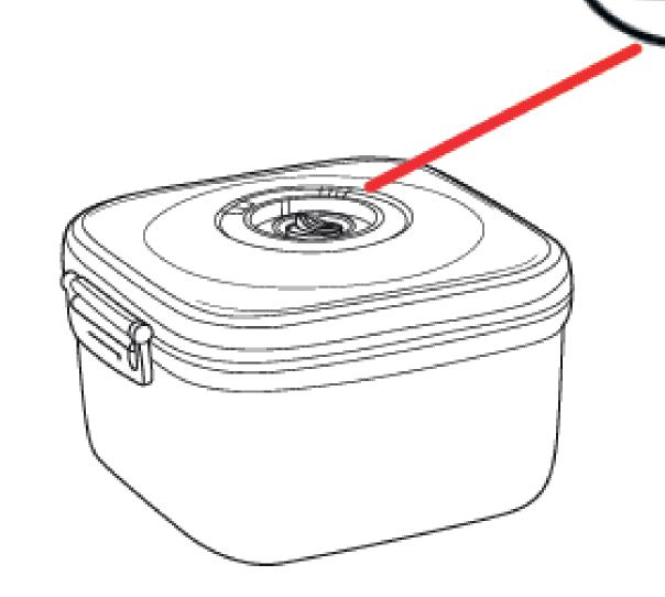
To release the vacuum from the container, please lift the air valve.
