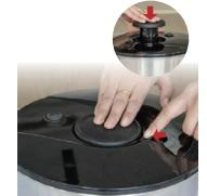
Lock the knob for space-saving. Push the knob down and hold it; then slide the knob lock inwards until it clicks into position.
