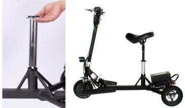
You can use included bungee cord to bundle a carry-on suitcase with the scooter while using travel seat. Hook one end of the bungee cord to the seat post support and through the rear bumper. Lay luggage flat on top of the battery and rear bumper. Tie the bungee cord around the luggage and hook the other end to the seat post support.
