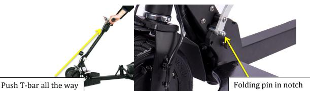
VERY IMPORTANT: Push the T-bar all the way forward and make sure the folding pin is fully seated in its notch. (You will hear a "click", which is the sound of folding pin hitting the bottom of the notch.
