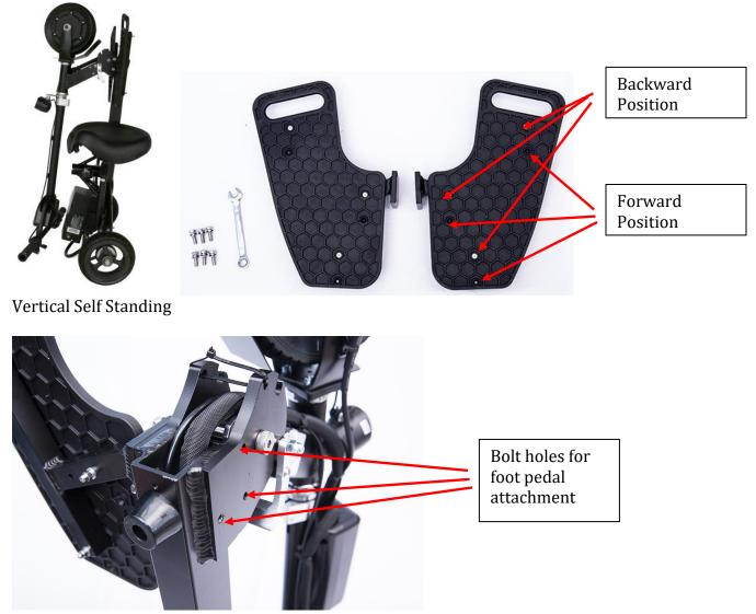
Step 2: Using the wrench, bolts and washers provided, attache the foot pedals to the flanges with the flat washer against the scooter frame and the lock washer between the flat washer and the bolt head.
