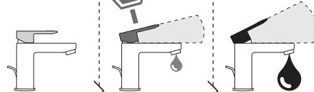
Closed position      Position of water saving "50% capacity"      100% Fully open flow
