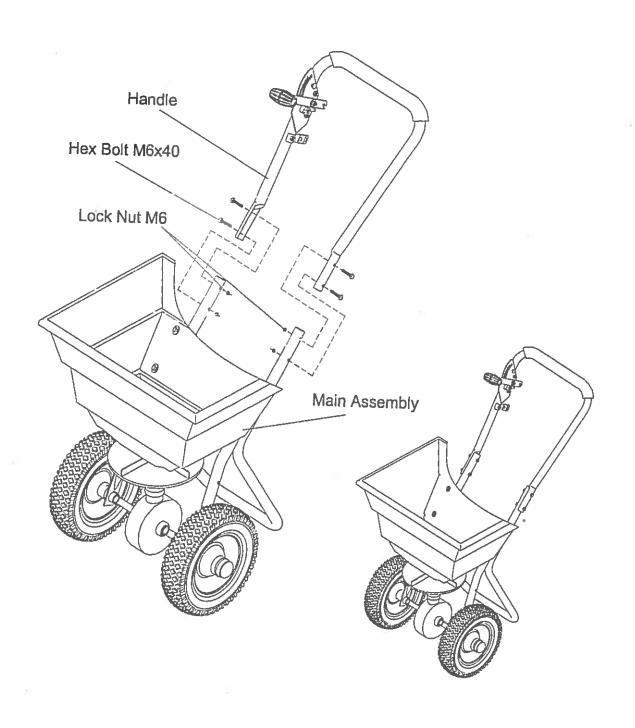
STEP 5: (1) Insert the steel wire into the adjustable handle pole. (2) Put the cable into the slot of pressure plate.(3)Screw on the bolt. (4) Insert R pin into the hole on small wheel shaft.
