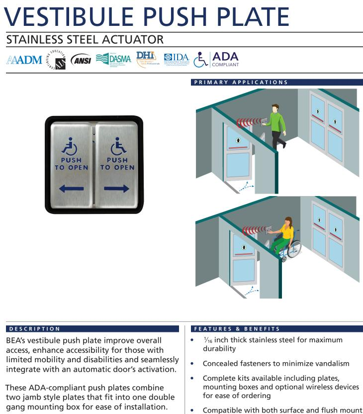
This push plates may be hard wired to the door operator or connected to BEA's line of wireless transmitters.
