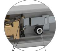
Roller bearings provide smooth operation of the touch bar
