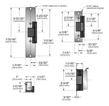
Solenoid power requirements; 12VDC, 0.38 A, 24 VDC, 0.19 A
