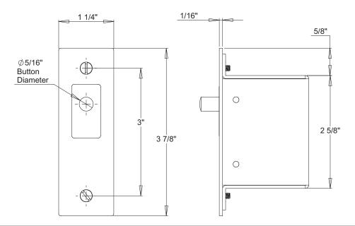
The door switch can be mounted to the switch case with the 2 flat head screws (supplied).
