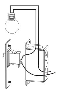
Contact rating- 10 Amps at 120 volts 5 Amps at 250 volts (DO NOT EXCEED CONTACT RATING)
