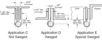
For all full mortise applications the center of barrel should be set 7/8" (22.2 mm) from door and frame so welded joints will clear. Leaves can be swaged apart any distance between 1/16" (1.6 mm) to 9/16" (14.3 mm)
