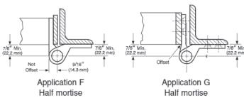
Variations of half mortise or half surface types can be obtained by further bumping or swaging of mortise leaf to accommodate any required construction. Specify hand when ordering
