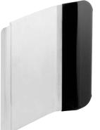
Designed for exterior doors that require extra security or resistance to vandalism, anti-vandal trim (AVT) plates have an extended lip on the active side of the door to provide extra protection for the latchbolt. A matte plastic coated grip provides a comfortable pull over wide temperature ranges. Fully through-bolted with no exposed exterior fasteners for a cleaner look and increased security.
