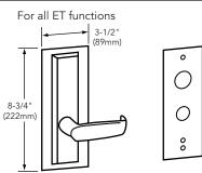
This plate is designed to be mounted behind the ET control to cover a stock hollow metal cutout
