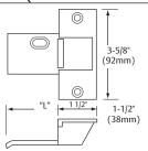
Full mortised dimension "L" equals door thickness plus 1/2" (13mm).
