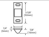
Half mortised. Nylon coating on face plate only. Minimum stile 4". When ordered separately, specify finish.
