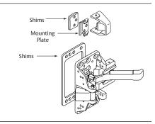
Half mortised. Nylon coating on face plate only. Minimum stile 4". When ordered separately, specify finish.
