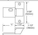
Full mortised Dimension "L" equals door thickness plus 1/2" (13mm).
