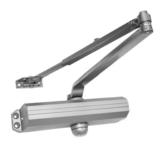
The RU package is provided with non hold open arm which includes additional bracket that allows installer the choice of standard, parallel or top jamb application. Used on Rated and Non Fire rated doors.
