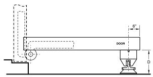
900 base has a minimum: 1-1/2" (38mm) extension. Maximum: 10" using combination of spacers [1/2" (13mm), 3/4" (19mm), etc.] Longer armature projections may encourage abuse and/or the weight of the extended rods will pull off the face of the door.
