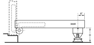
900 base has a minimum: 1-1/2" (38mm) extension. Maximum: 10" using combination of spacers [1/2" (13mm), 3/4" (19mm), etc.] Longer armature projections may encourage abuse and/or the weight of the extended rods will pull off the face of the door.
