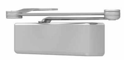
The 4110 is LCN's best performing heavy duty closer with an adjustable spring and possible hold open point beyond 140 degrees, meeting ADA requirements. Backed by a 30 year warranty, the cast iron body and all weather fluid offer versatility in high traffic applications.
