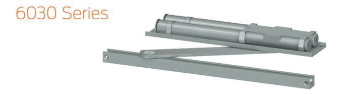
The concealed 6030 Series PACER® is a heavy duty double acting closer designed to fit in a narrow, minimum 1 3/4" header. The single lever arm and roller assembly provides smooth, quiet door control and the choice of finishes and track functions meet virtually all architectural requirements.
