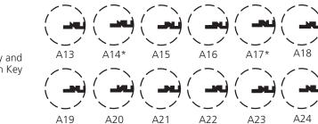
\* NOTE: Do not use these pairs in the same keying system with each other: A13 with A14; A16 with A17.
