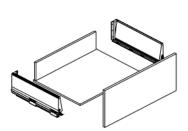
8 Install the drawer rail fitting on the board by using screws
