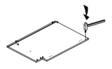
Keep a side panel flat on the floor, then insert bottom panel
