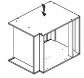
5 Put the screw into the screw hole
