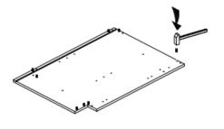
2 Keep a side panel flat on the floor, then insert bottom panel
