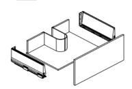
8 Install the drawer rail fittings on the board by using screws
