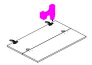
9 Put the hinge into the base, then install doors
