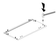
2 Keep a side panel flat on the floor, then insert top panel
