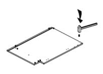
Keep a side panel flat on the floor, then insert bottom panel
