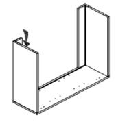
8 Install the hinge base on the side panel
