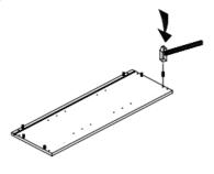
2 Keep a side panel flat on the floor, then put the top panel on
