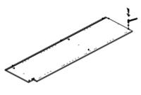
Keep a side panel flat on the floor, then insert top&bottom panels and shelf
