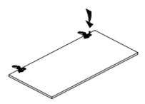
10 Put the hinges into the base, then install doors
