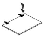
9 Put theb hinge into the base, then install doors
