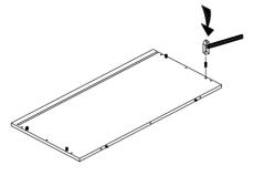
Keep a side panel flat on the floor, then insert top and bottom panel
