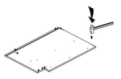
Keep a side panel flat on the floor, then insert bottom panel
