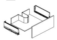
8 Install the drawer rail fittings on the board by using screws
