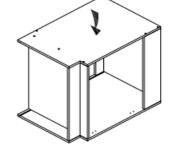
5 Put the screw into the screw hole
