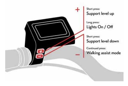
Finally, to turn on your front and rear light, press and hold the + button for 2 seconds.
